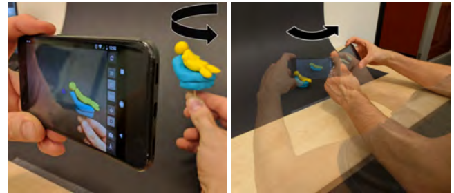
(a) Designer rotates the Play-Doh in front of the camera (b) Designer moves the camera around the Play-Doh in an orbit
