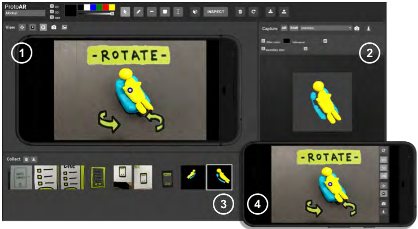
Figure 5. ProtoAR consists of two main interfaces: the ProtoAR Editor for laptop and the ProtoAR App for phone. The editor consists of three main components: (1) the view pane showing a live preview of the AR interface also shown on the phone, (2) the capture pane providing interactive capture tools to filter colors and crop the image, (3) the collect pane showing a collection of digitized 2D/3D objects that can be inserted into the view. (4) The app shows the AR interface streamed from the laptop and provides access to some editor functions.
